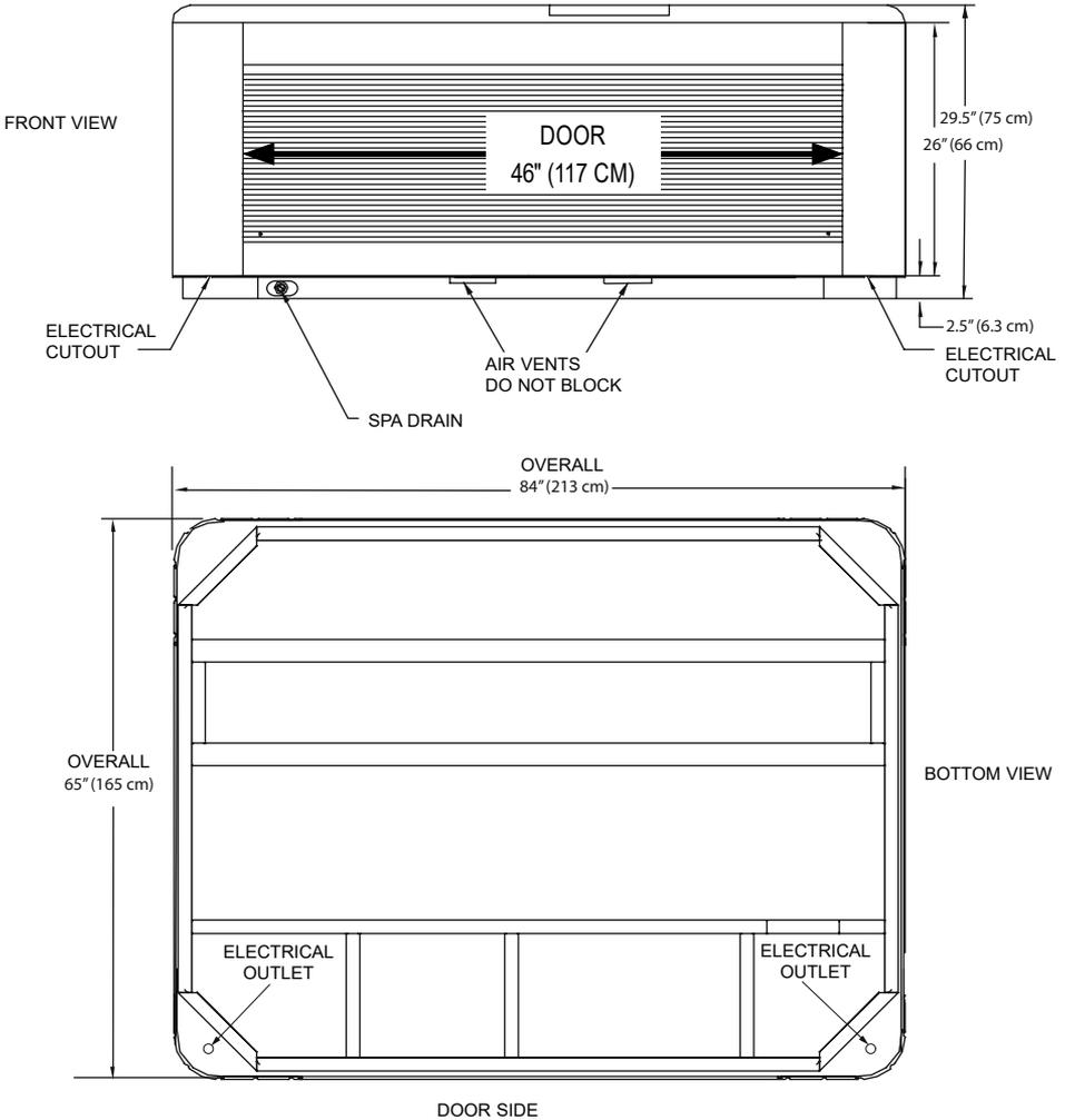
**NOTE: WATKINS WELLNESS** recommends that the Kauai be installed on a minimum 4" (10 cm) thick reinforced concrete pad or structurally sound deck able to support the "dead weight" found in the spa specification chart.
