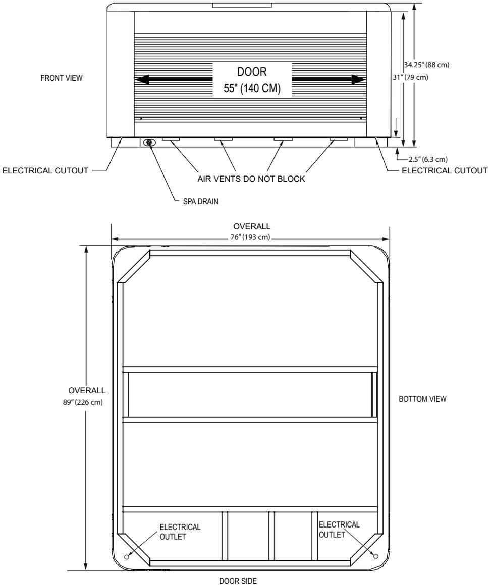
**NOTE: WATKINS WELLNESS** recommends that the Martinique be installed on a minimum 4" (10 cm) thick reinforced concrete pad or structurally sound deck able to support the "dead weight" found in the spa specification chart.
