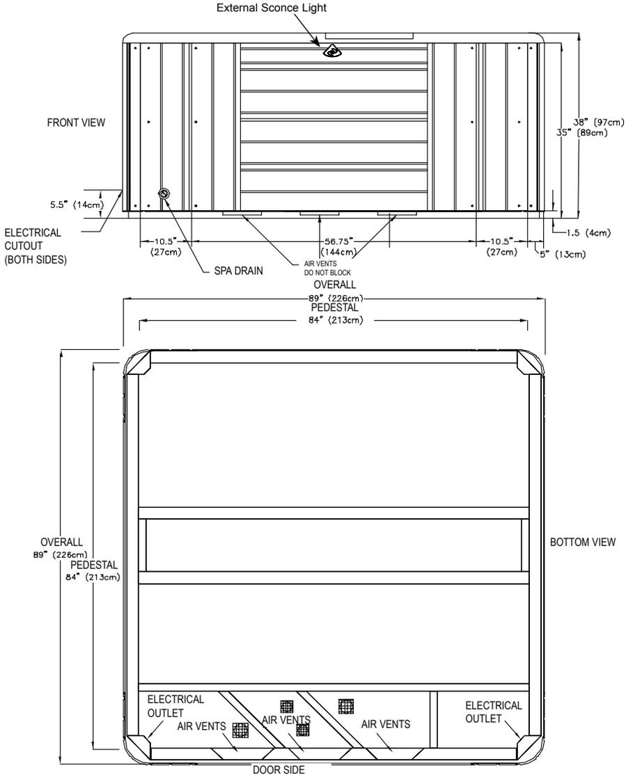
**NOTE:** Watkins Manufacturing Corporation requires that the Geneva and Niagara be installed on a minimum 4" thick reinforced concrete pad or structurally sound deck able to support the "dead weight" found in the spa specification chart.
