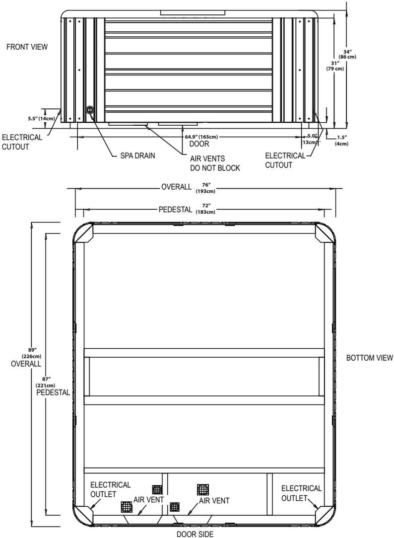
**NOTE:** Watkins Manufacturing Corporation recommends that the Martinique be installed on a minimum 4" thick reinforced concrete pad or structurally sound deck able to support the "dead weight" found in the spa specification chart.
