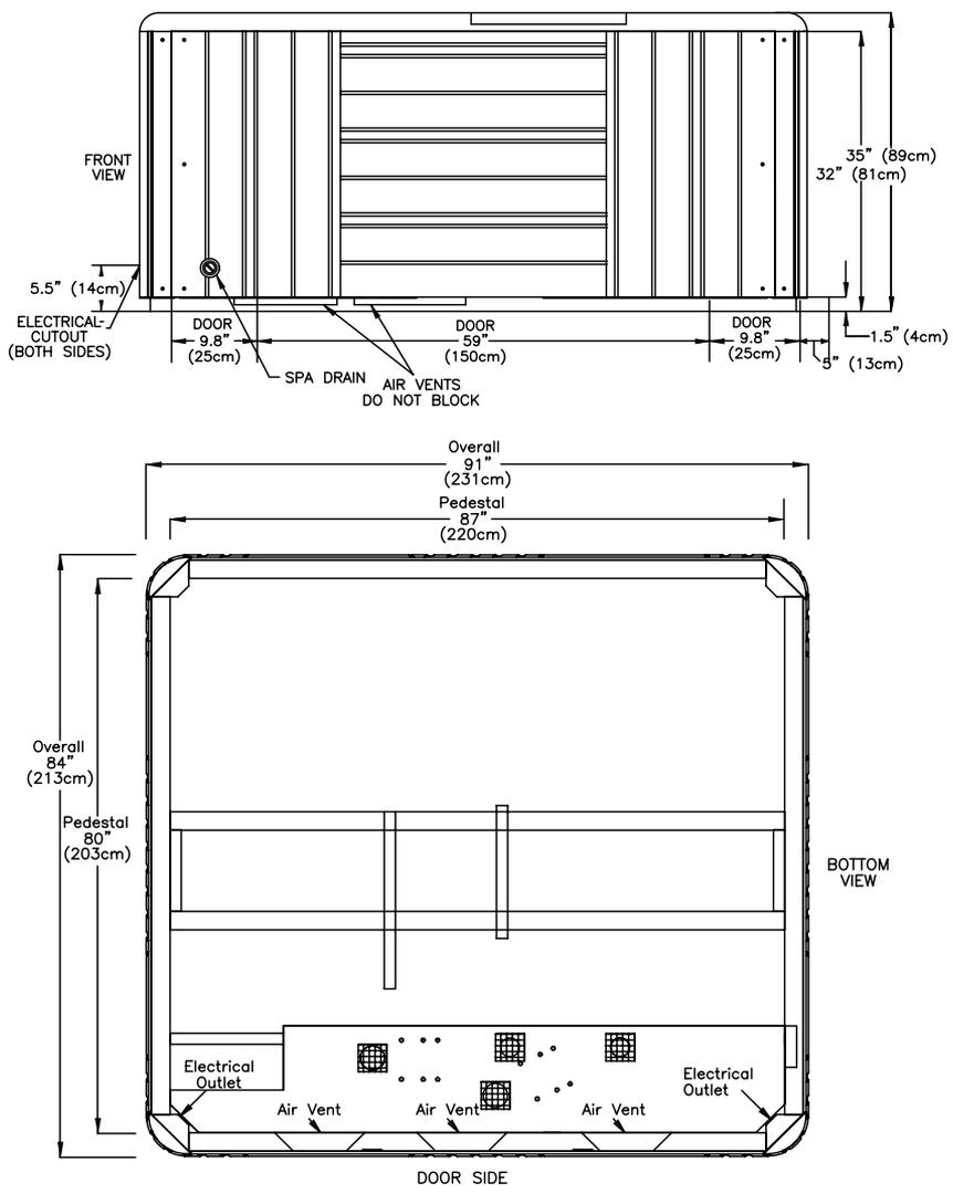
**NOTE:** Watkins Manufacturing Corporation requires that the Moorea be installed on a minimum 4" thick reinforced concrete pad or structurally sound deck able to support the "dead weight" found in the spa specification chart.
