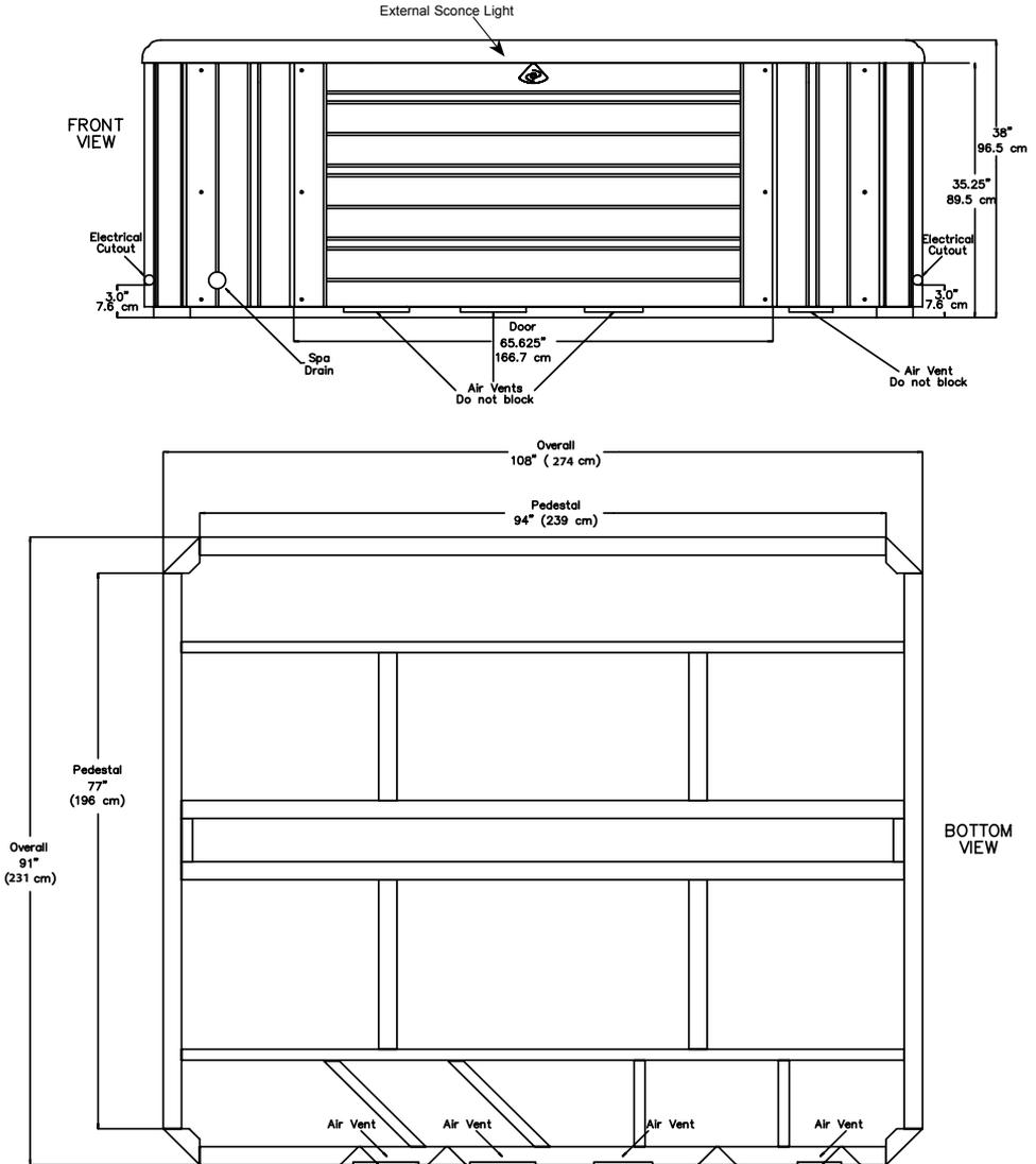
**NOTE:** Watkins Manufacturing Corporation requires that the Cantabria be installed on a minimum 4" thick reinforced concrete pad or structurally sound deck able to support the "dead weight" found in the spa specification chart.
