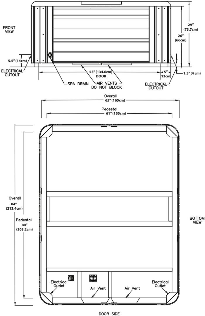
**NOTE:** Watkins Manufacturing Corporation recommends that the Kauai be installed on a minimum 4" thick reinforced concrete pad or structurally sound deck able to support the "dead weight" found in the spa specification chart.
