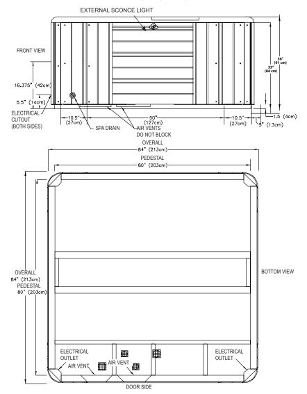
**NOTE:** Watkins Manufacturing Corporation recommends that the Tahitian be installed on a minimum 4" thick reinforced concrete pad or structurally sound deck able to support the "dead weight" found in the spa specification chart.
