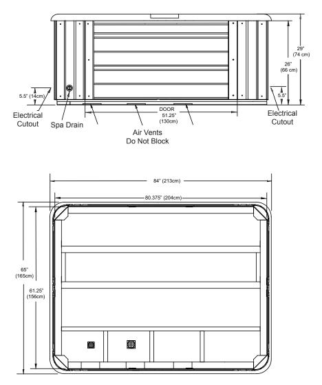
**NOTE:** Watkins Manufacturing Corporation recommends that the Kauai be installed on a minimum 4" thick reinforced concrete pad or structurally sound deck able to support the "dead weight" found in the spa specification chart.
