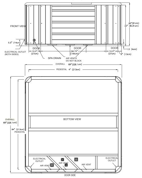
**NOTE:** Watkins Manufacturing Corporation requires that the Salina be installed on a minimum 4" thick reinforced concrete pad or structurally sound deck able to support the "dead weight" found in the spa specification chart. **WARNING:** The Salina must not be shimmed in any manner.
