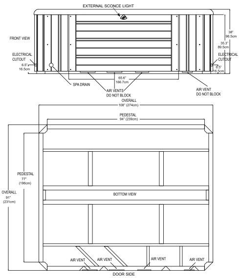
NOTE: Watkins Manufacturing Corporation requires that the Cantabria be installed on a minimum 4" thick reinforced concrete pad or structurally sound deck able to support the "dead weight" found in the spa specification chart. WARNING: The Cantabria must not be shimmed in any manner.
