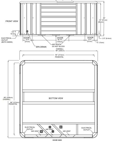
**NOTE:** Watkins Manufacturing Corporation requires that the Salina be installed on a minimum 4" thick reinforced concrete pad or structurally sound deck able to support the "dead weight" found in the spa specification chart.
