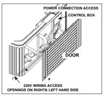
**IMPORTANT:** The following must be followed to properly install the equipment compartment door.
