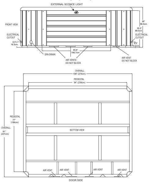
NOTE: Watkins Manufacturing Corporation requires that the Cantabria be installed on a minimum 4" thick reinforced concrete pad or structurally sound deck able to support the "dead weight" found in the spa specification chart. WARNING: The Cantabria must not be shimmed in any manner.
