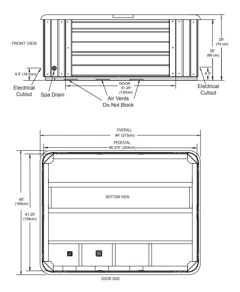
**NOTE:** Watkins Manufacturing Corporation recommends that the Kauai be installed on a minimum 4" thick reinforced concrete pad or structurally sound deck able to support the "dead weight" found in the spa specification chart. **WARNING:** The Kauai must not be shimmed in any manner.
