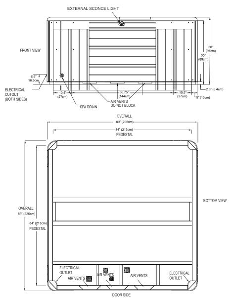
**NOTE:** Watkins Manufacturing Corporation requires that the Geneva and Niagara be installed on a minimum 4" thick reinforced concrete pad or structurally sound deck able to support the "dead weight" found in the spa specification chart. **WARNING:** The Geneva and Niagara must not be shimmed in any manner.
