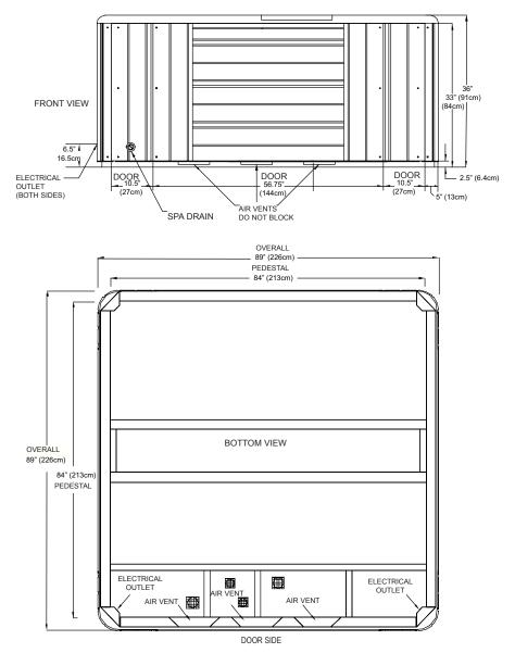
**NOTE:** Watkins Manufacturing Corporation requires that the Makena and Salina be installed on a minimum 4" thick reinforced concrete pad or structurally sound deck able to support the "dead weight" found in the spa specification chart.
