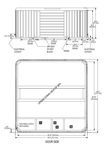
**NOTE:** Watkins Manufacturing Corporation recommends that the **MARINO** & **VANTO** be installed on a minimum 4" (10 cm) thick reinforced concrete pad or structurally sound deck able to support the "dead weight" found in the spa specification chart.
