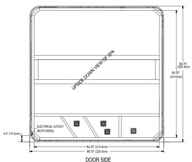
**NOTE:** Watkins Manufacturing Corporation recommends that the **PALATINO** be installed on a minimum 4" (10 cm) thick reinforced concrete pad or structurally sound deck able to support the "dead weight" found in the spa specification chart.
