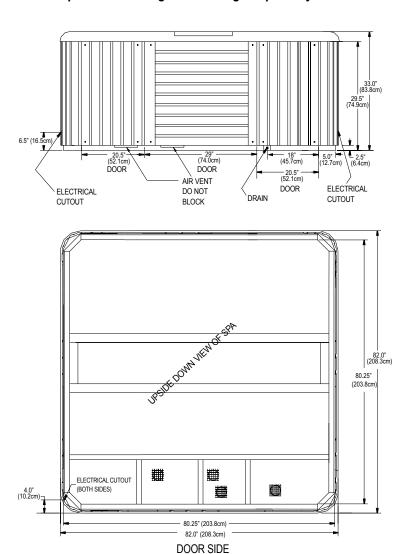
**NOTE:** Watkins Manufacturing Corporation recommends that the **TARINO** be installed on a minimum 4" (10 cm) thick reinforced concrete pad or structurally sound deck able to support the "dead weight" found in the spa specification chart.
