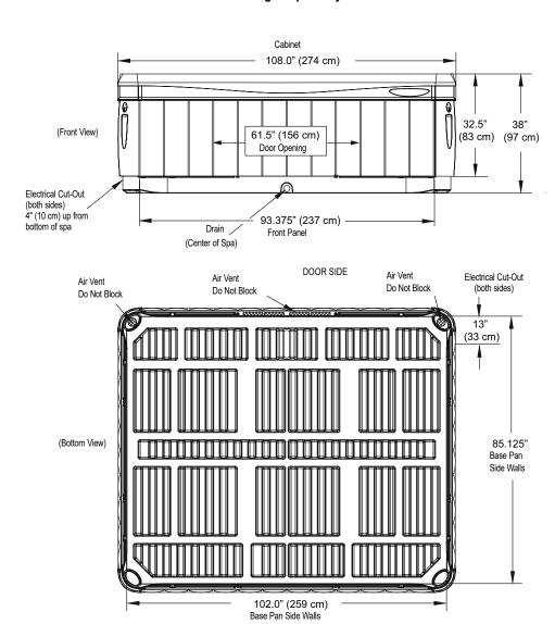
NOTE: Watkins Manufacturing Corporation requires that the **CANTABRIA** be installed on a minimum 4" (10 cm) thick reinforced concrete pad or structurally sound deck able to support the "dead weight" found in the spa specification chart.
