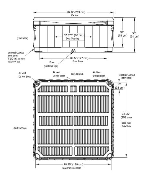
**NOTE:** Watkins Manufacturing Corporation recommends that the **TAHITIAN** be installed on a minimum 4" thick reinforced concrete pad or structurally sound deck able to support the "dead weight" found in the spa specification chart.
