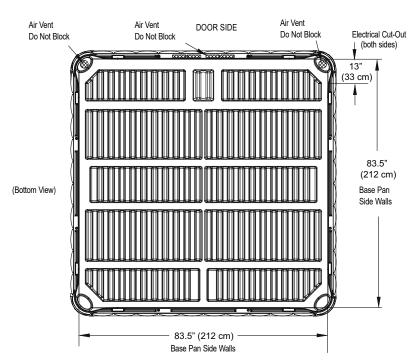
**NOTE:** Watkins Manufacturing Corporation requires that the **GENEVA** and **NIAGARA** be installed on a minimum 4" thick reinforced concrete pad or structurally sound deck able to support the "dead weight" found in the spa specification chart.
