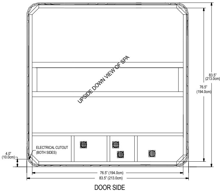
**NOTE:** Watkins Manufacturing Corporation recommends that the **MARINO & VANTO** be installed on a minimum 4" (10 cm) thick reinforced concrete pad or structurally sound deck able to support the "dead weight" found in the spa specification chart.
