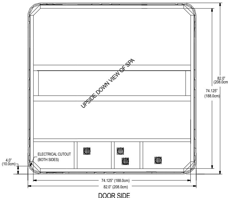
**NOTE:** Watkins Manufacturing Corporation recommends that the **TARINO** be installed on a minimum 4" (10 cm) thick reinforced concrete pad or structurally sound deck able to support the "dead weight" found in the spa specification chart.
