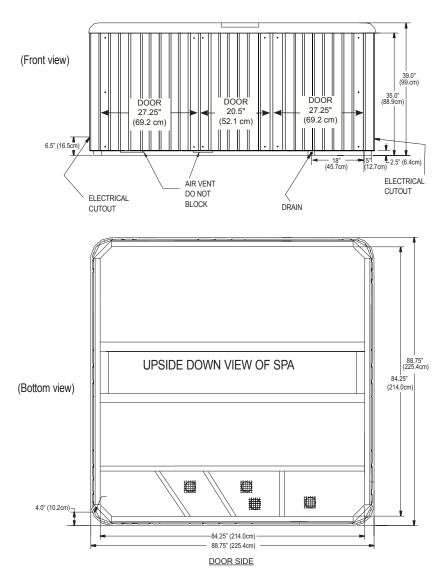
**NOTE: WATKINS WELLNESS** recommends that the Tempo be installed on a minimum 4" (10.2 cm) thick reinforced concrete pad or structurally sound deck able to support the "dead weight" found in the spa specification chart.
