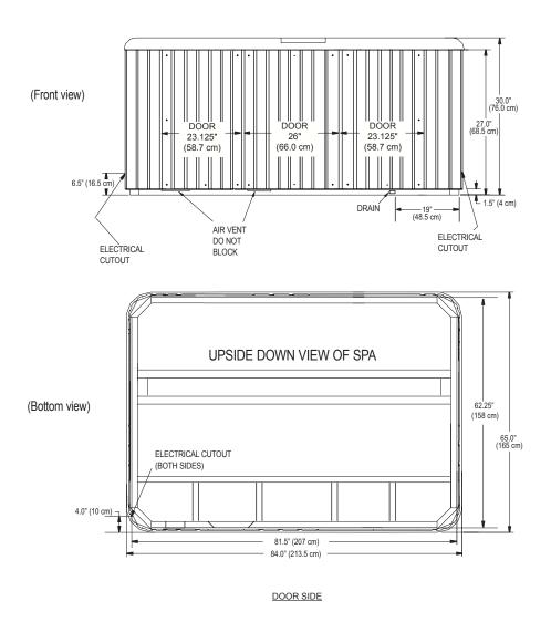
**NOTE: WATKINS WELLNESS** recommends that the Stride be installed on a minimum 4" (10.2 cm) thick reinforced concrete pad or structurally sound deck able to support the "dead weight" found in the spa specification chart. **IMPORTANT:** THE STRIDE MUST NOT BE SHIMMED IN ANY MANNER.
