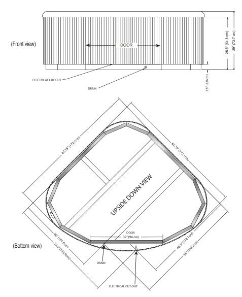
**NOTE: WATKINS WELLNESS** recommends that the TX be installed on a minimum 4" (10.2 cm) thick reinforced concrete pad or structurally sound deck able to support the "dead weight" found in the spa specification chart. **IMPORTANT:** THE TX MUST NOT BE SHIMMED IN ANY MANNER.
