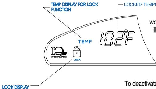
To activate the TEMPERATURE LOCK, press the LIGHT plus (+) and TEMP plus (+) buttons at the same time and hold them down until the words SET TEMP, the numerical set temperature value and the lock symbol are illuminated on the display (approximately 2 seconds).
