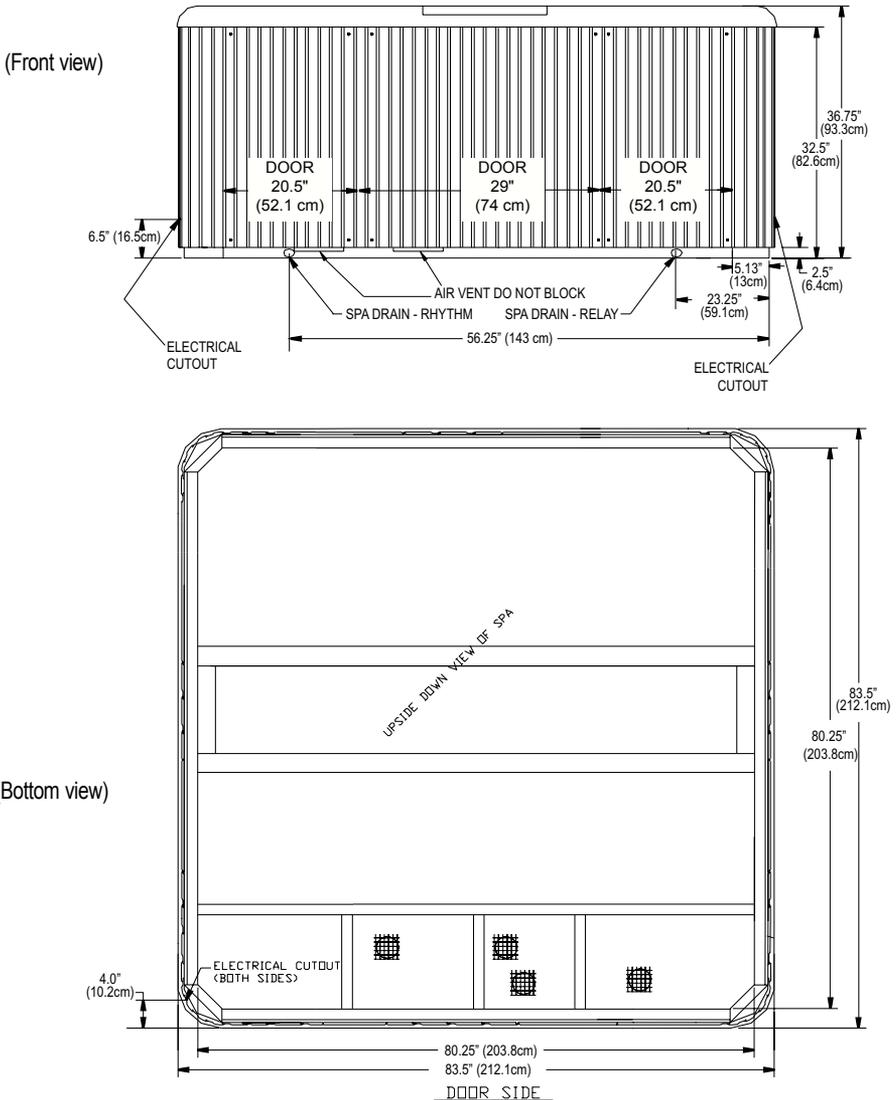
**NOTE:** Watkins Manufacturing Corporation recommends that the Relay & Rhythm be installed on a minimum 4" (10.2cm) thick reinforced concrete pad or structurally sound deck able to support the "dead weight" found in the spa specification chart.
